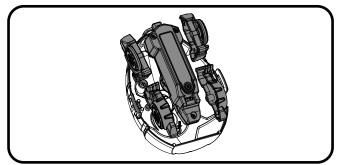
Place the battery module and the 4 dino legs into the egg shell as illustrated.
